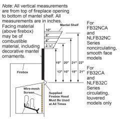
Figure 7 - Minimum Mantel Clearances for Built-In Installation
